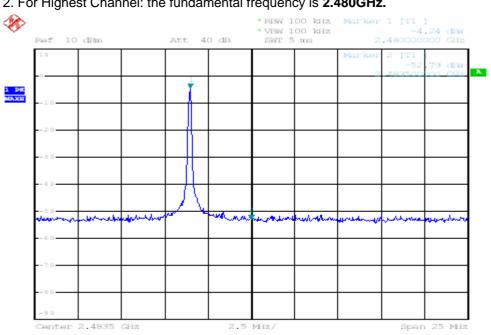
2. For Highest Channel: the fundamental frequency is 2.480GHz.
