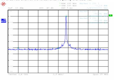
1. For Lowest Channel: the fundamental frequency is 2.402G Hz.
