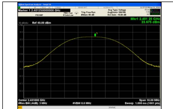
Low Channel – Peak Conducted Output Power
