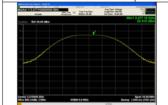
High Channel – Peak Conducted Output Power
