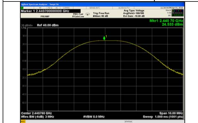
Middle Channel – Peak Conducted Output Power
