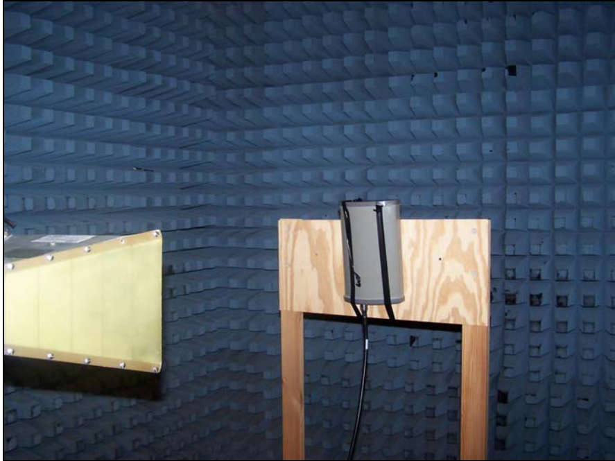
Photograph 5. Spurious Radiated Emissions, Test Setup, 120° 9 dBi Sector
