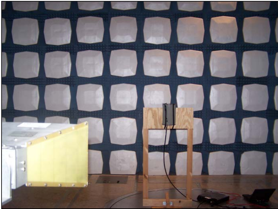
Photograph 2. Band Edge, 120° 9 dBi Sector, Test Setup
