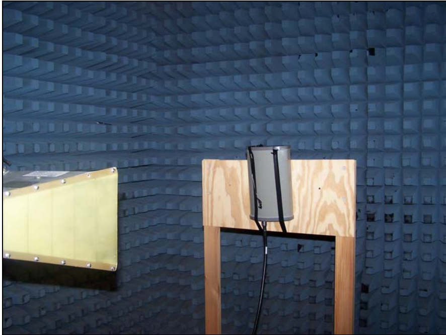
Photograph 5. Spurious Radiated Emissions, Test Setup, 120° 9 dBi Sector
