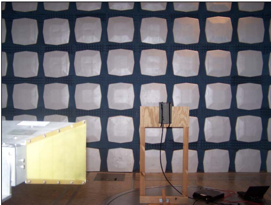
Photograph 2. Band Edge, 120° 9 dBi Sector, Test Setup
