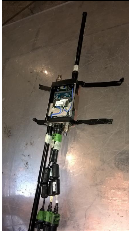
Photograph 5. Radiated Emissions Below 1 GHz, Modification to Support Equipment 5
