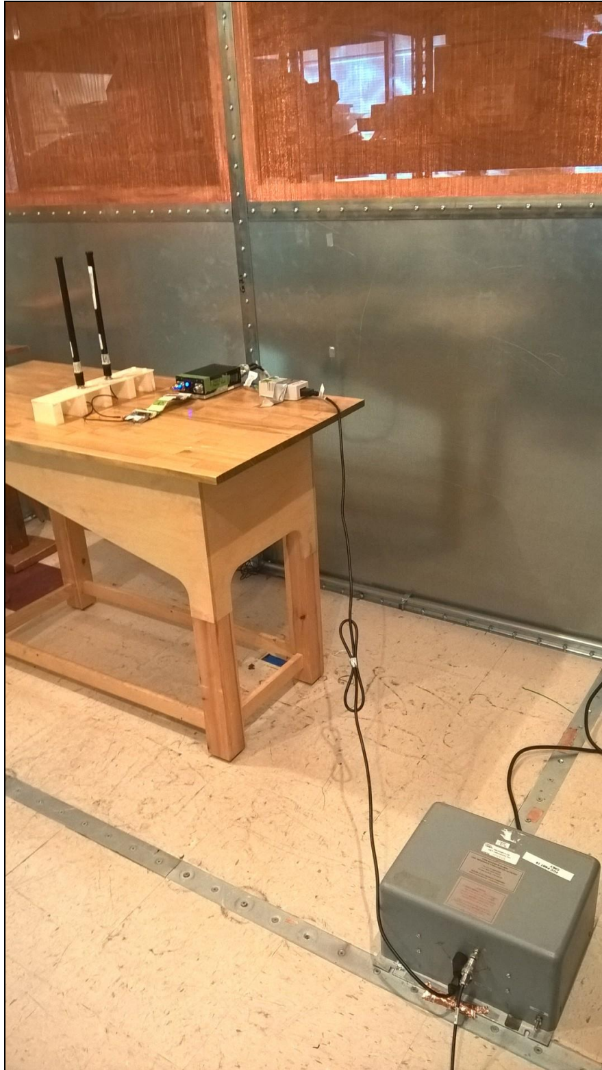
Photograph 7. Conducted Emissions, Test Setup
