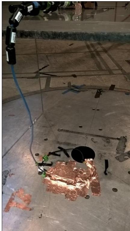
Photograph 4. Radiated Emissions Below 1 GHz, Modification to Support Equipment 4
