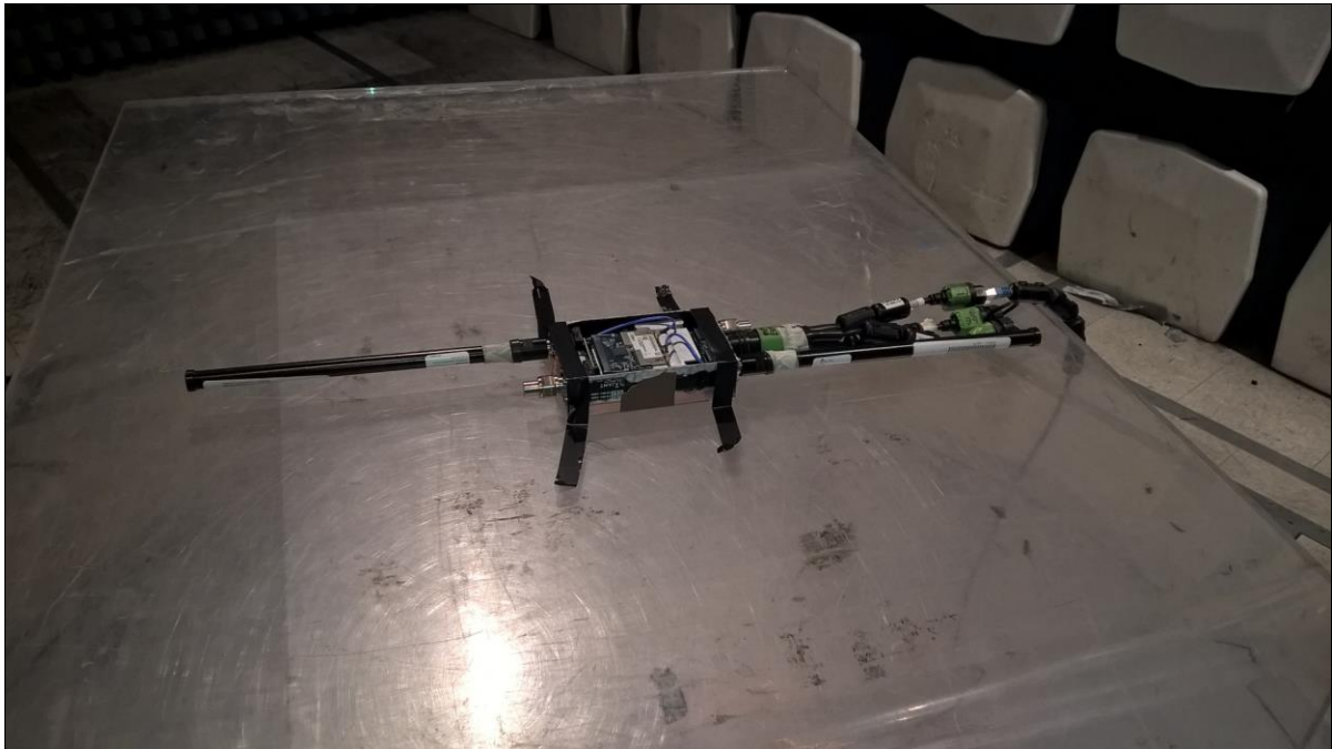
Photograph 1. Radiated Emissions Below 1 GHz, Modification to Support Equipment 1
