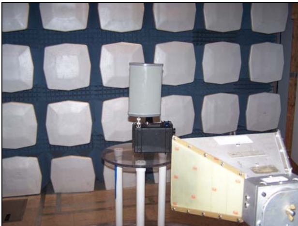
Photograph 2. Spurious Radiated Emissions Test Setup, 9 dBi Sector
