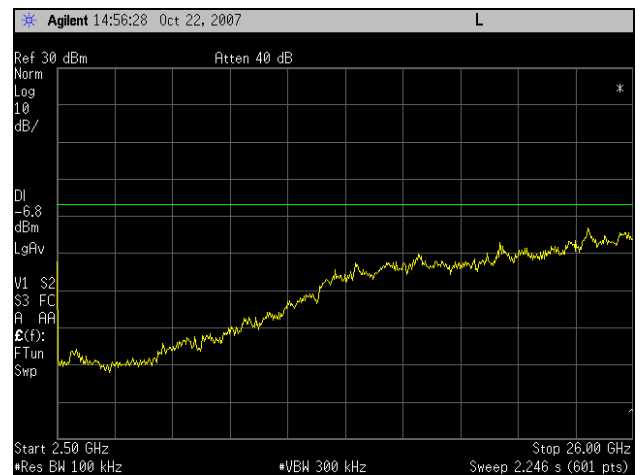
Spurious RF Conducted Emissions, Channel 11, 2.5GHz – 26GHz
