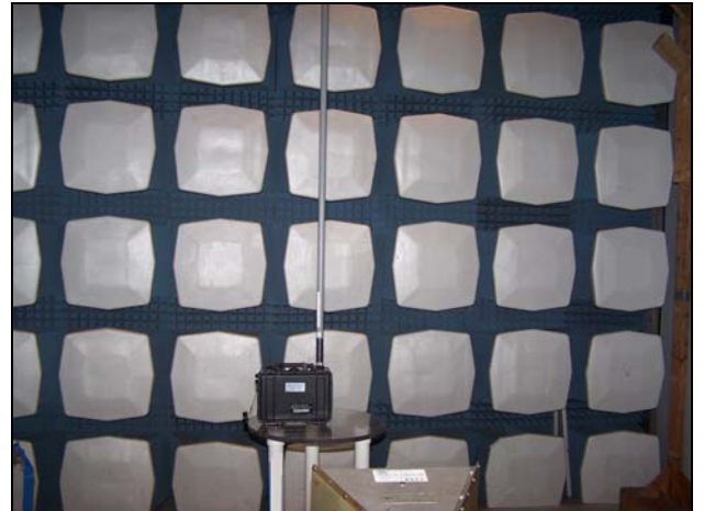
Photograph 3. Spurious Radiated Emissions Test Setup, 12 dBi Omni
