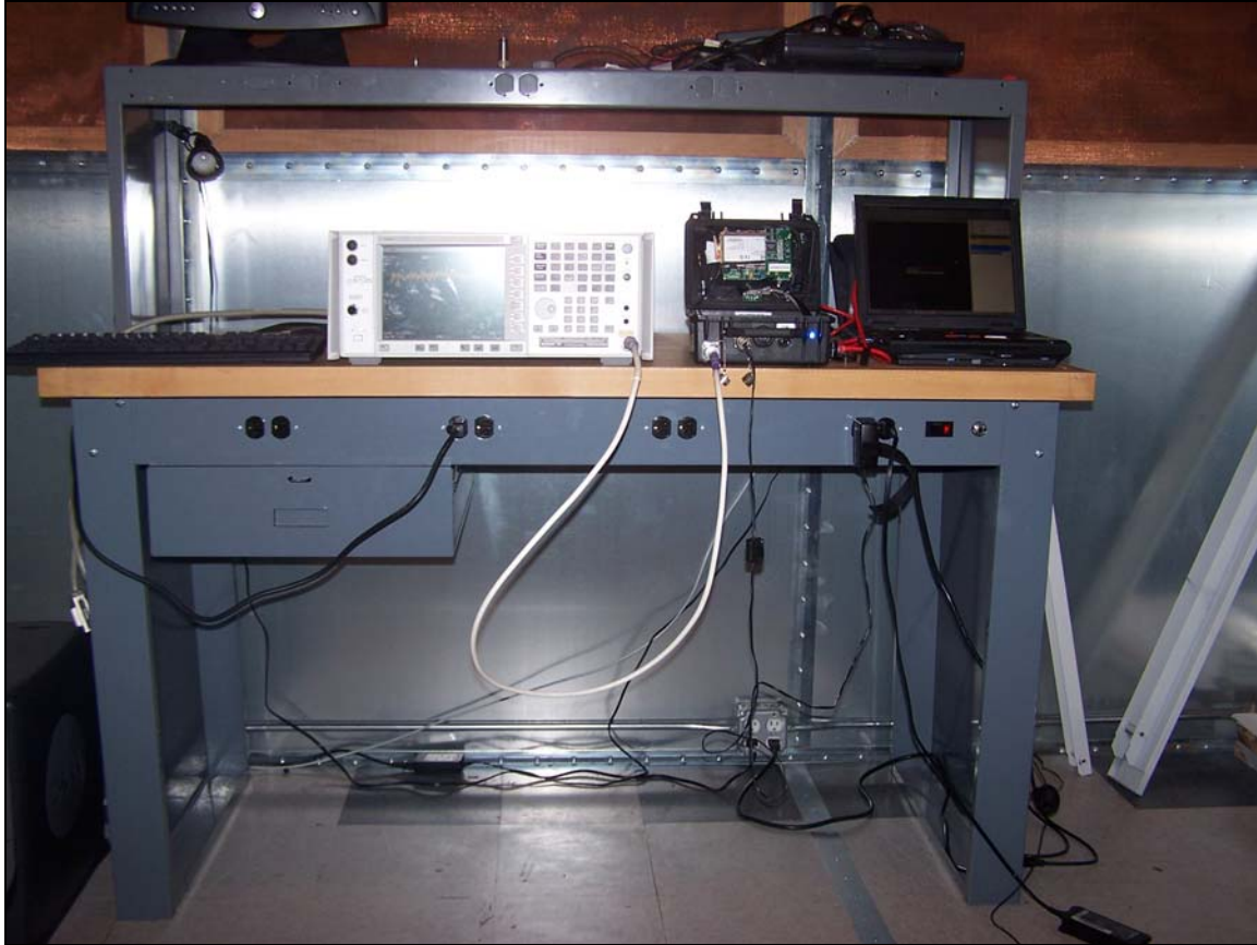
Photograph 6. 6 dB Bandwidth Test Setup
