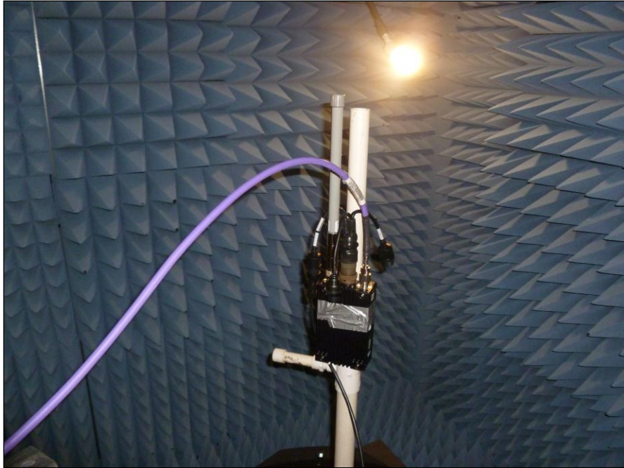
Photograph 5. Peak Power Output, Test Setup, 2.4 GHz
