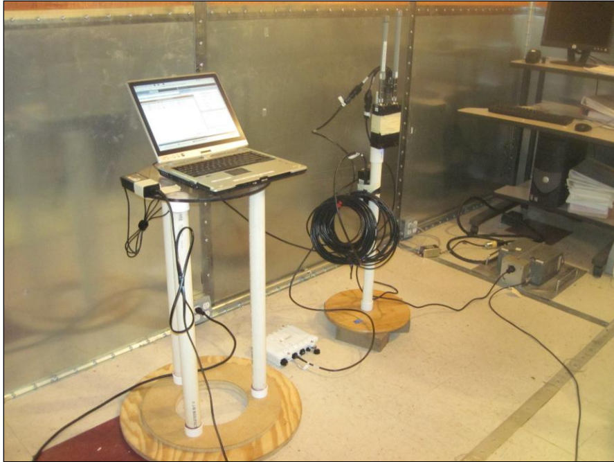
Photograph 3. Conducted Emissions, 15.207(a), Test Setup, 2.4 GHz
