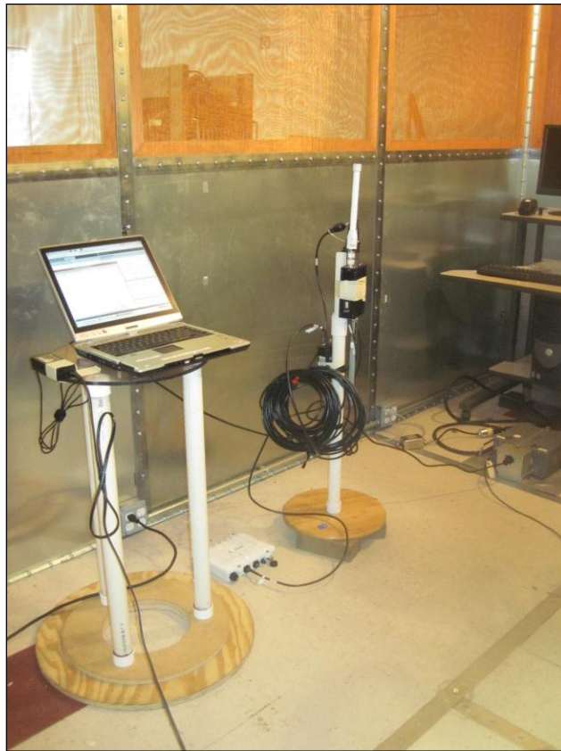
Photograph 4. Conducted Emissions, 15.207(a), Test Setup, 5 GHz
