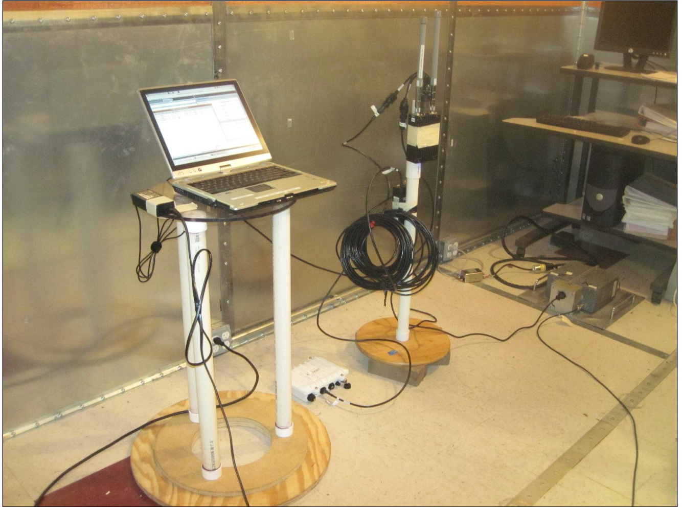
Photograph 4. Conducted Emissions, 15.207(a), Test Setup
