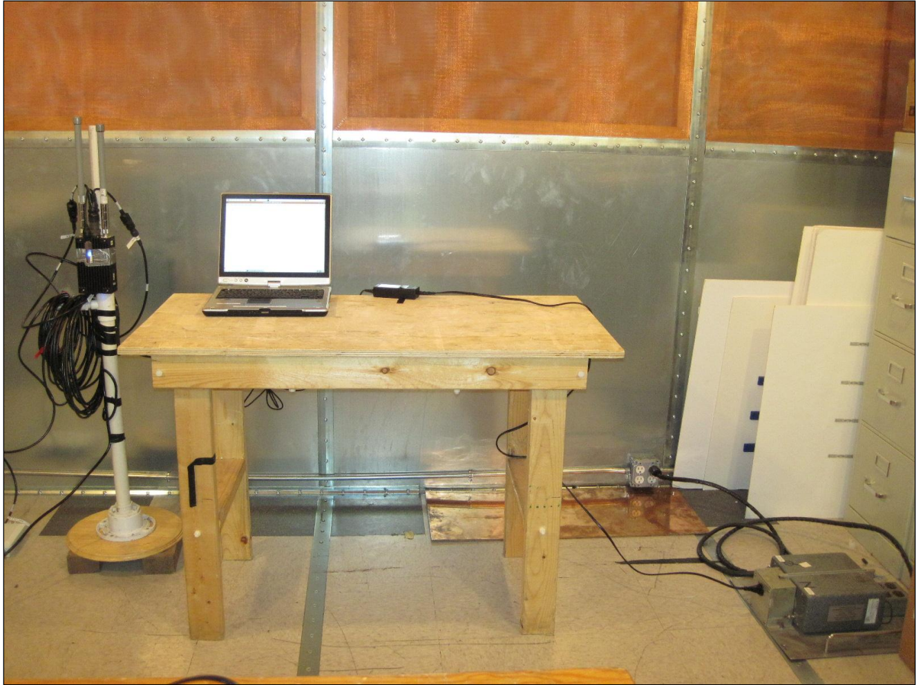
Photograph 1. Conducted Emissions, Test Setup
