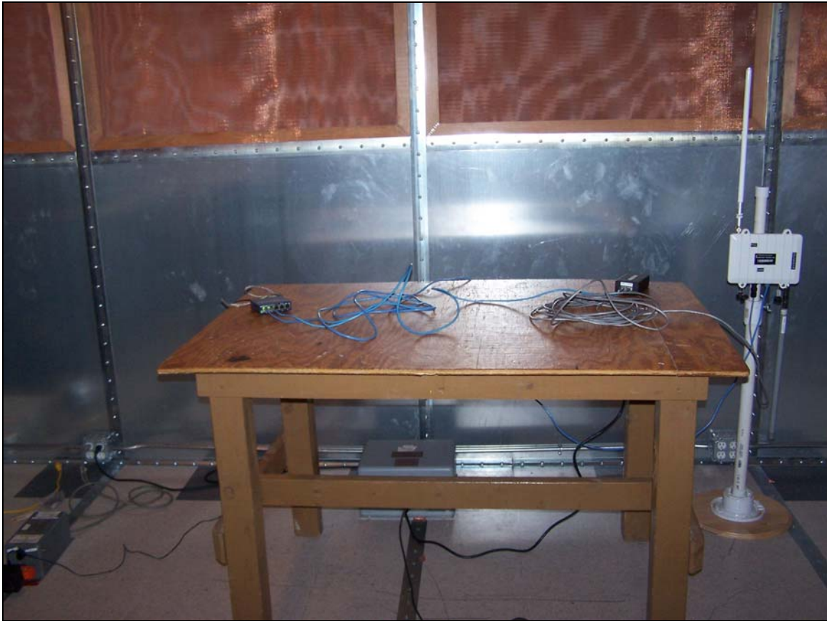
Photograph 3. Conducted Emissions, Test Setup
