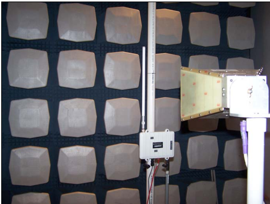
Photograph 5. Radiated Emission Test Setup, 5.8 GHz Mode
