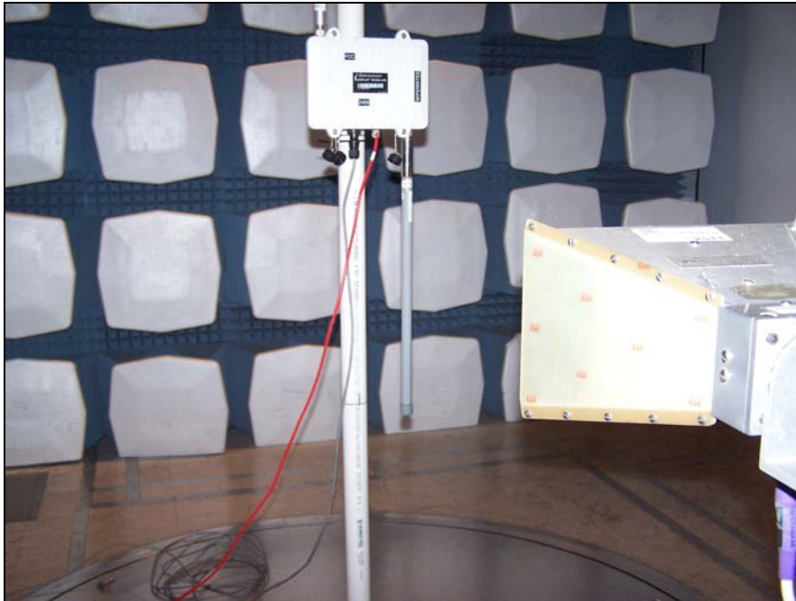
Photograph 4. Radiated Emission Test Setup, b and g Mode, 2.4 GHz
