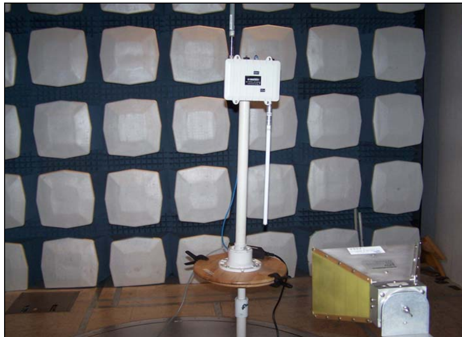
Photograph 2. Restricted Band Test Setup, 5.8 GHz
