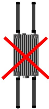
Figure: Incorrect Antenna Placement (ME4 shown)
