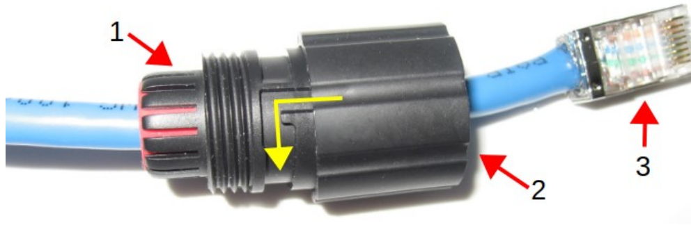
Figure: Lining Up and Mating Inner and Outer Shells
