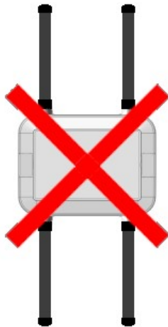
Figure: Incorrect Antenna Placement
