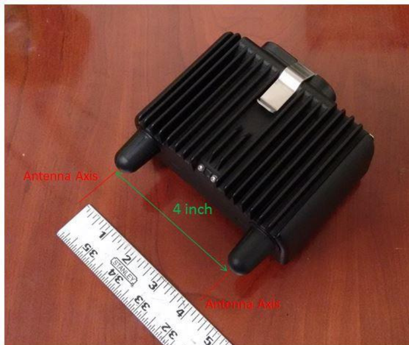
Figure 4. Rajant CX1-3600 with antenna separation illustrated
