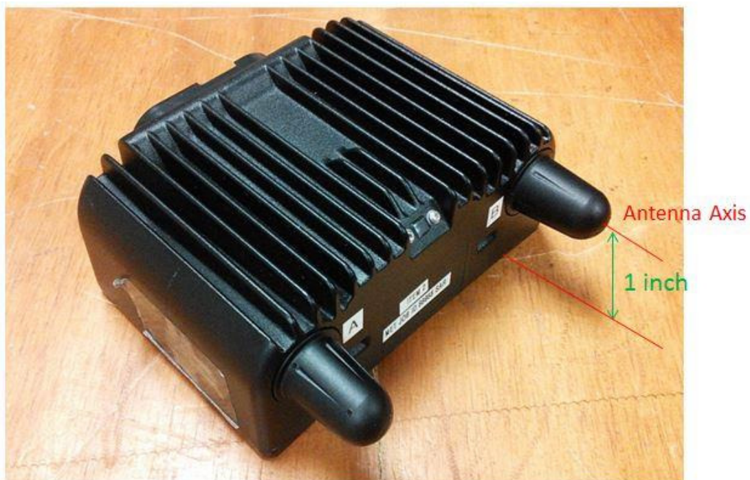
Figure 5. Rajant CX1-3600 with antenna separation illustrated
