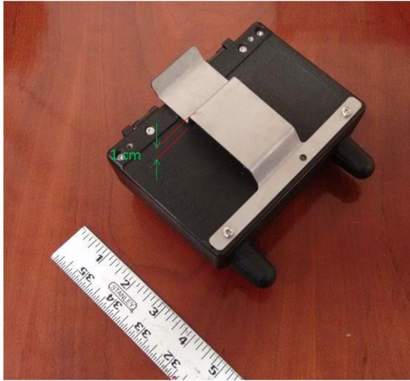
Figure 25. EUT with belt clip separation illustrated
