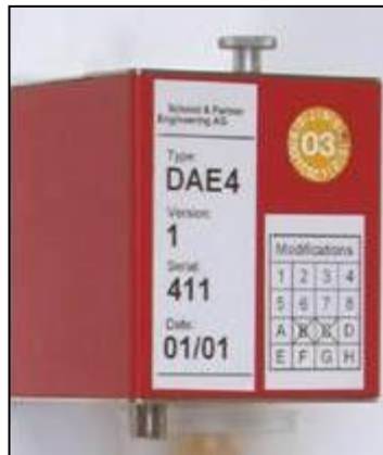
Figure 15. Data acquisition electronics.
