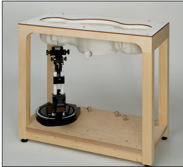
Figure 19. Specific anthropomorphic mannequin twin phantom
