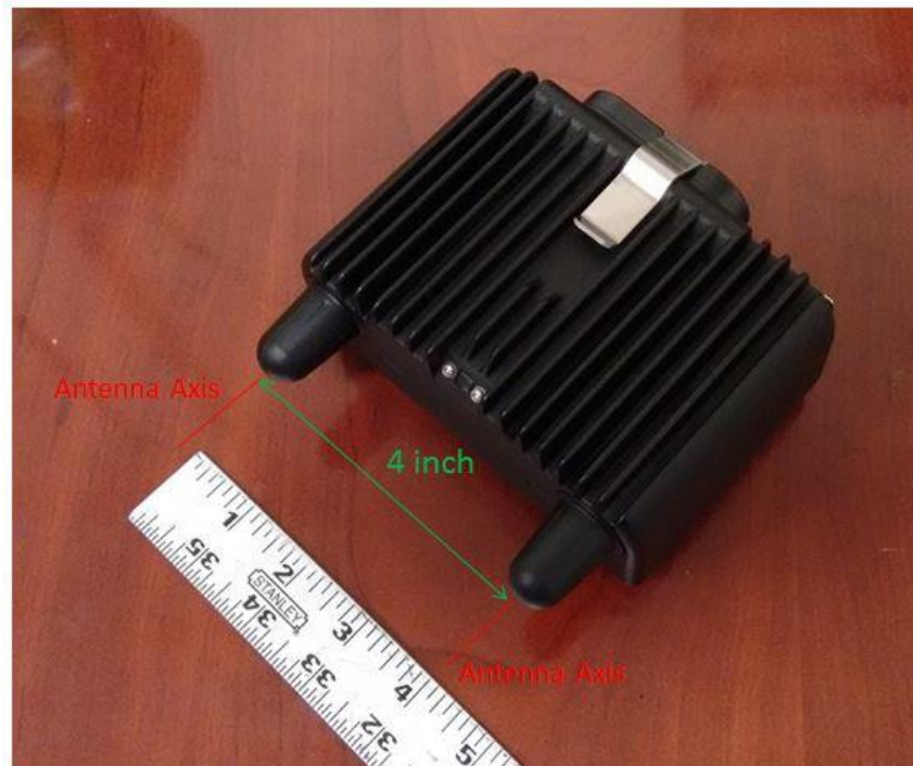
Figure 4. Rajant CX1-3600 with antenna separation illustrated
