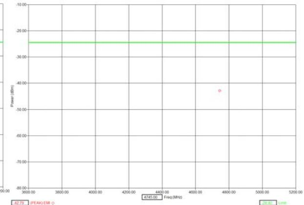
Measurements made with 3 MHz RBW / 3 MHz VBW at 3 meter distance.
