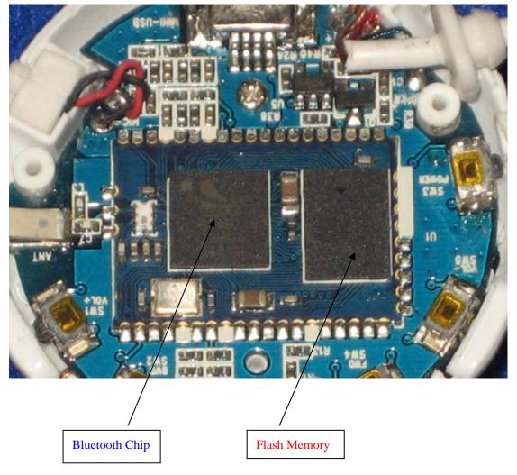
From the above photo, we can see that the Bluetooth chip and flash memory are located on a small rectangle PWB defined as U1 which has 50pins.
