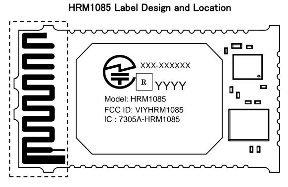
The label is printed with a laser on a shield case.
