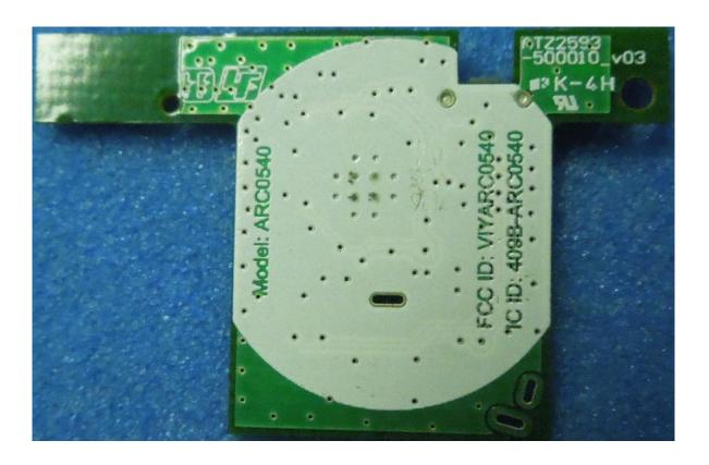
Following IDs are displayed inside of red square area (backside of PWB) with silk printing.
