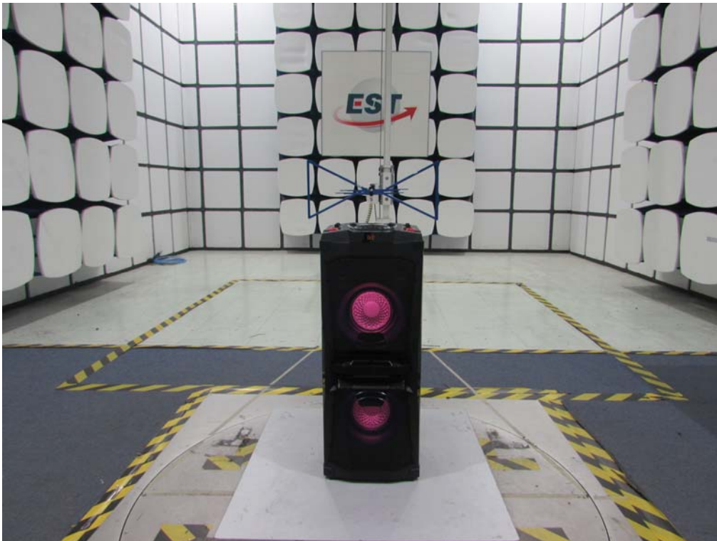
Radiated Test (30-1000 MHz)
