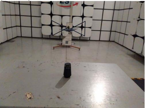
Radiated Test (1000-25000 MHz)
