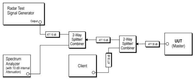
Remark: During the test, a lower radar signal level -64dBm was used.
