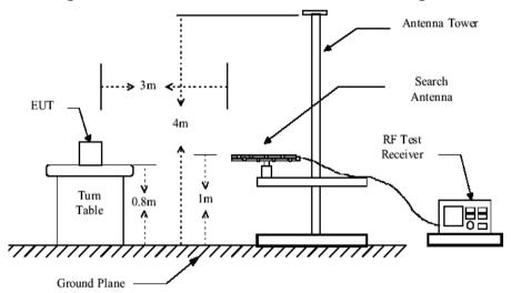
Figure 2. 30MHz to 1GHz radiated emissions test configuration
