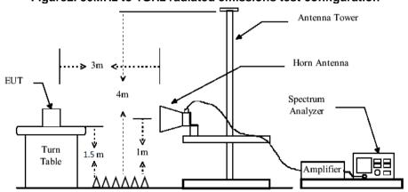
Figure 3. Above 1GHz radiated emissions test configuration
