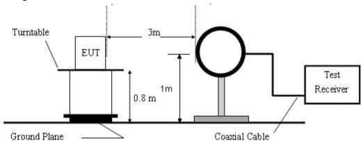
Figure 1. Below 30MHz radiated emissions test configuration
