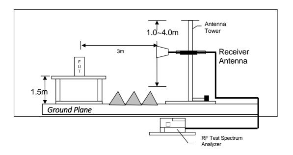
Test setup of radiated emissions above 1GHz
