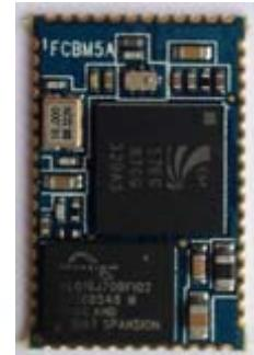
The ZYM-BT55 module is a power class2 Bluetooth® device, and is in compliance with version 2.1 of the Bluetooth® specification. It includes CSR BC05 MultiMedia Core and 8Mbit/16Mbit/32Mbit Flash memory, a radio front-end, antenna interface, supporting circuitry, together with some higher-level software protocols and applications such as L2CAP, SDP, GAP, HSP, HFP, A2DP, AVRCP, OPP and PBAP resided in the flash memory.
