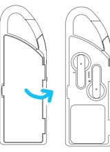
Insert the provided charging cable into the charging jack on the side of the speaker. Plug the other end of the charging cable into a USB power source (like a computer or a USB charger).
