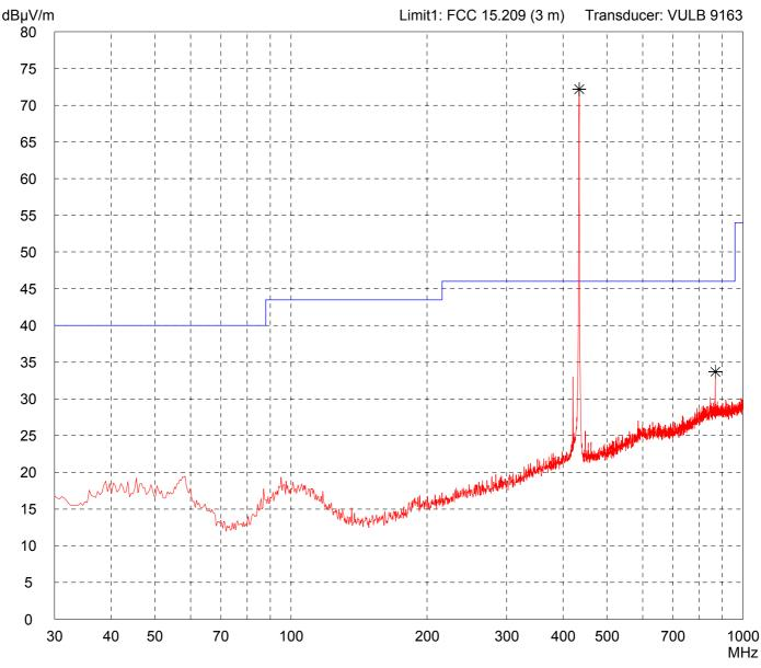
Model: PD remote control (Porsche Design) Applicant: **EMV-Testhaus GmbH** Fully anechoic room, cabin no. 2 Tested on: Test distance 3 metres Vertical Polarization Date of test: Operator: 07/06/2007 M. Steindl File name: Test performed: automatically default.emi
