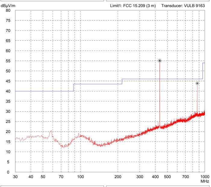
Model: PD remote control (Porsche Design) Applicant: **EMV-Testhaus GmbH** Fully anechoic room, cabin no. 2 Tested on: Test distance 3 metres Vertical Polarization Date of test: Operator: 07/06/2007 M. Steindl File name: Test performed: automatically default.emi
