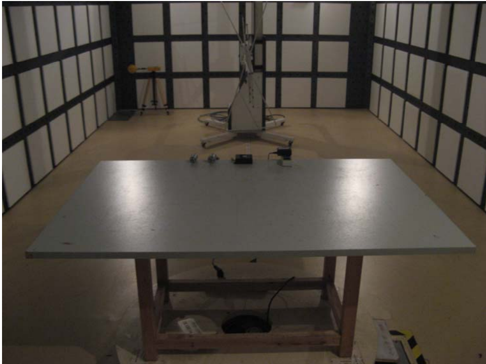
FCC RADIATED EMISSION TEST SETUP
