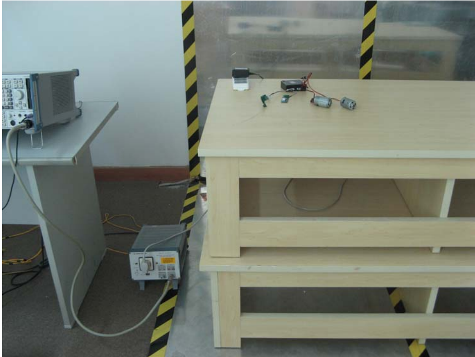
FCC RADIATED EMISSION TEST SETUP
