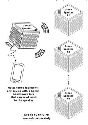
The Control Speaker can be connected to any analog device with the 3.5mm stereo plug cable supplied. Then the Control Speaker can link to the Drone Speaker(s).
