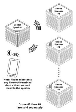
This is the typical setup for multiple speakers connected to the Control Speaker. If there are no Drone Speakers connected the Control acts like a single bluetooth speaker.
