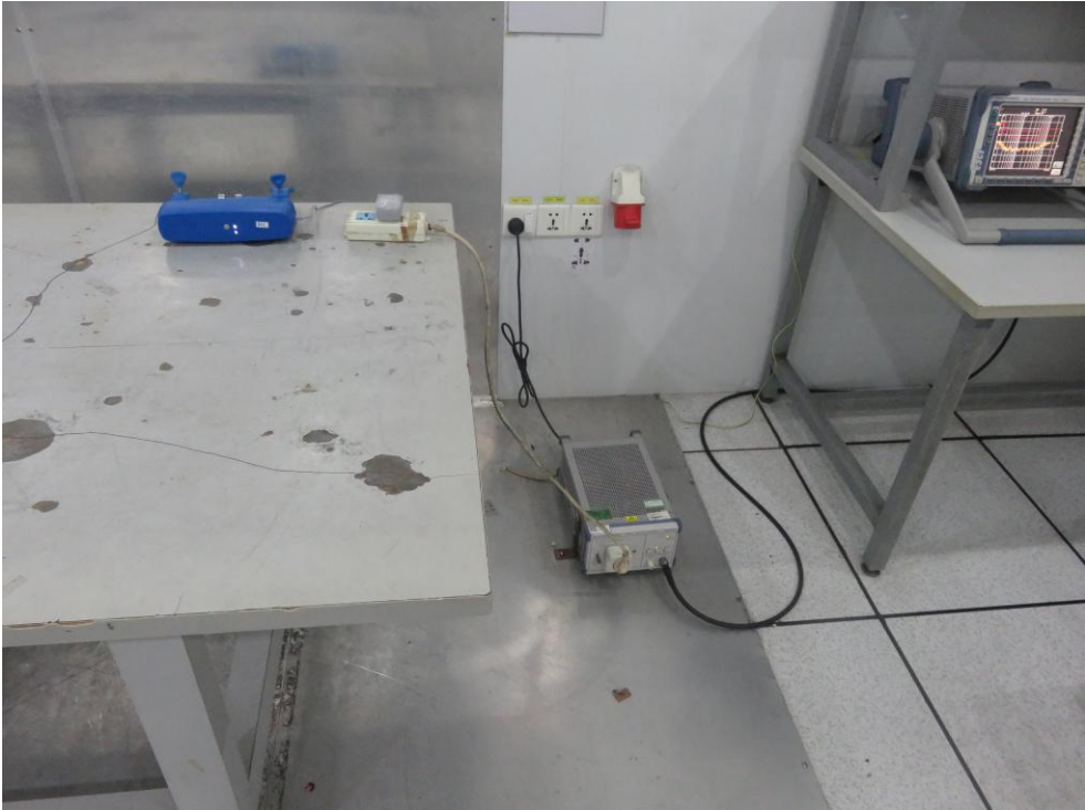
Photo of Conducted Emission Test
