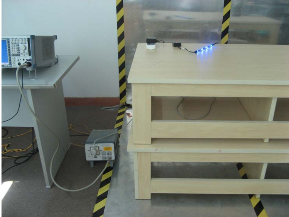
FCC RADIATED EMISSION TEST SETUP
