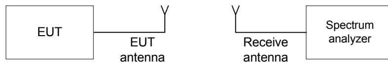
Figure 7.7.1 Band edge emission test setup
