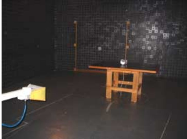
Photograph No.5 Setup for radiated emission measurements in the anechoic chamber above 1000 MHz
