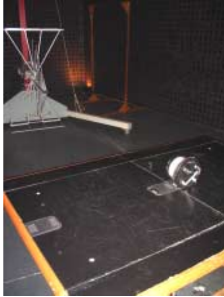
Photograph No.1 Setup for carrier field strength measurements and OBW in the anechoic chamber
