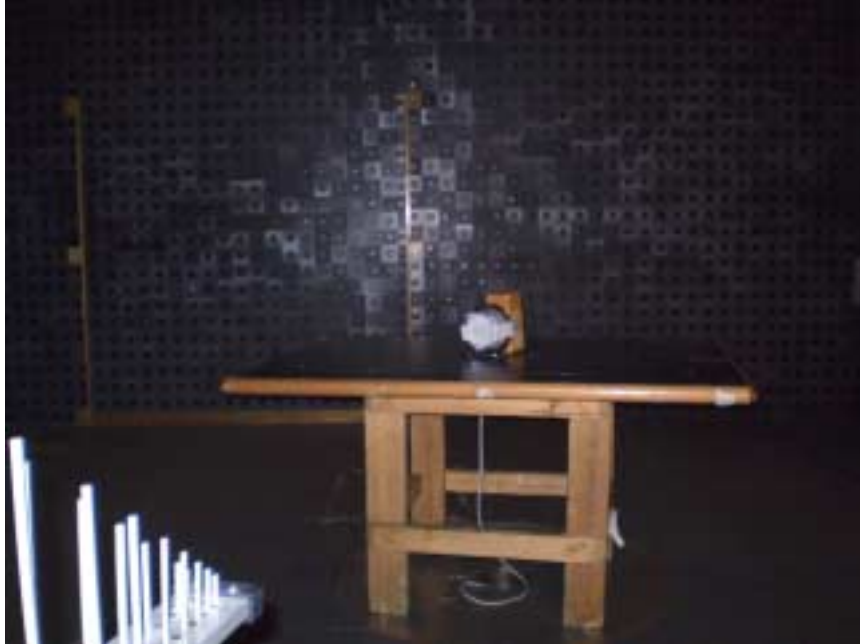
Photograph No.3 Setup for radiated emission measurements in the anechoic chamber from 30 to 1000 MHz
