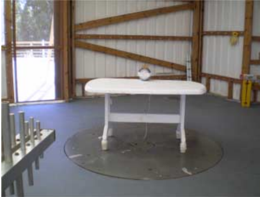
Photograph No.1 Setup for carrier field strength, peak spectral power density and OBW measurements at the OATS
