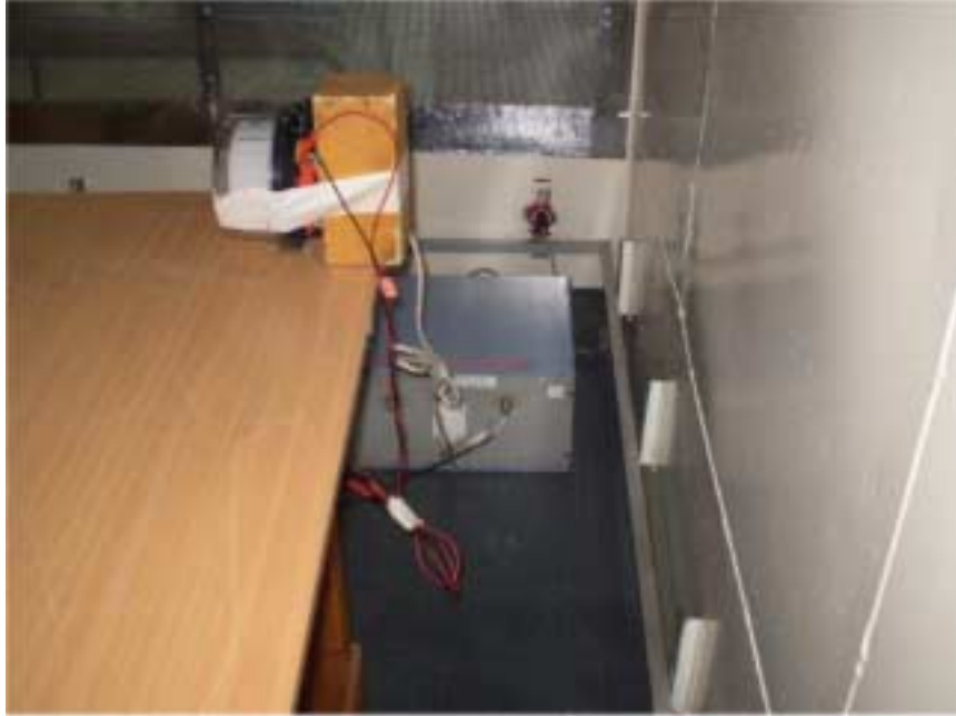
Photograph No.6 Setup for conducted emission measurements on the EUT power ports
