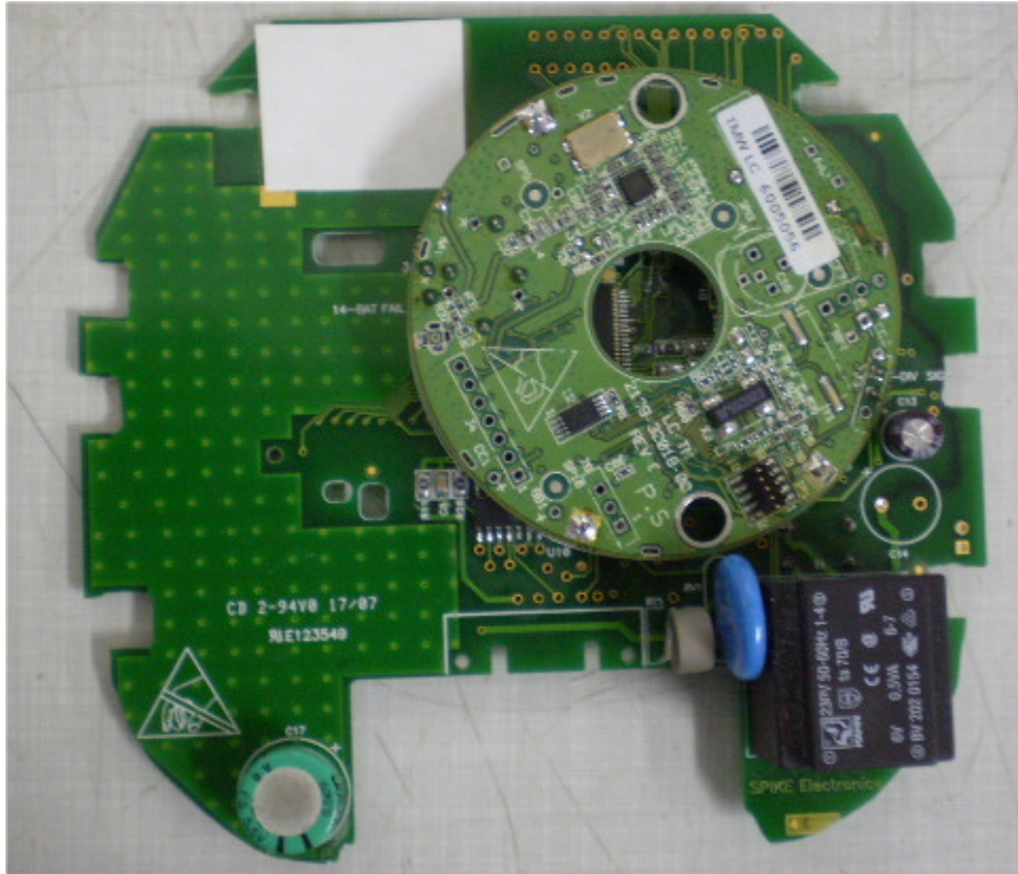
Photograph No.8 Display board view from the second side with RF module (antenna closed)
