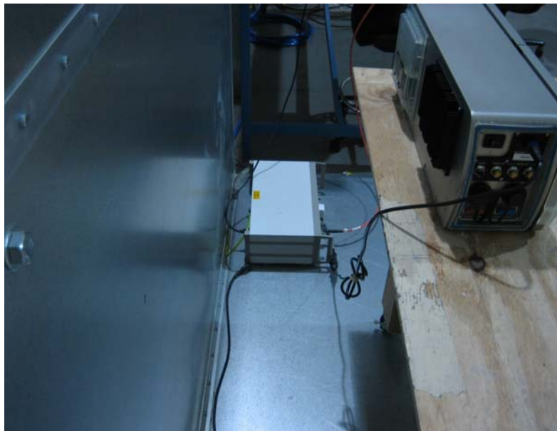
AC Line Conducted Emission Test Set-up Rear View
