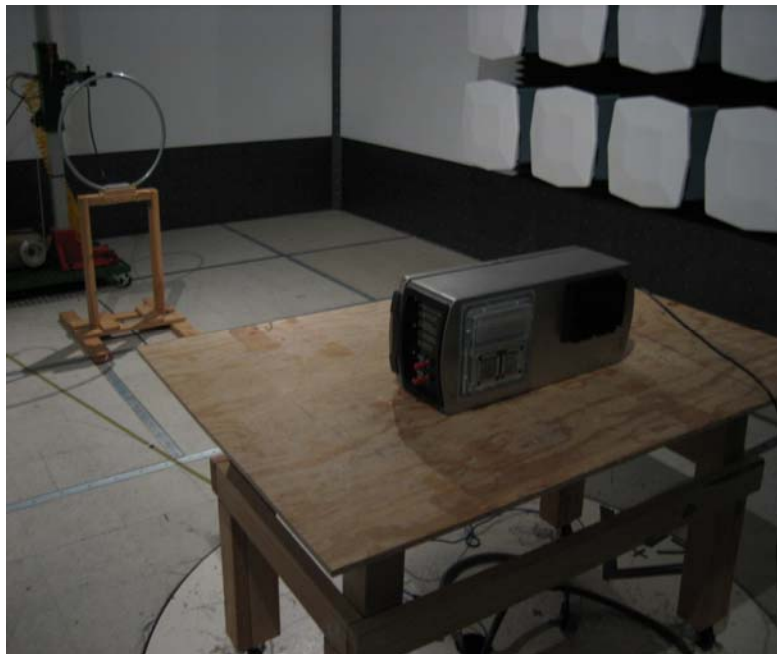
Radiated Emission Test Set-up Rear View ( < 30 MHz )
