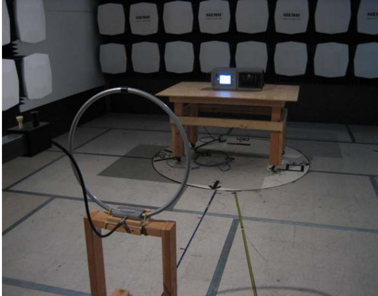
Radiated Emission Test Set-up Front View ( < 30 MHz )
