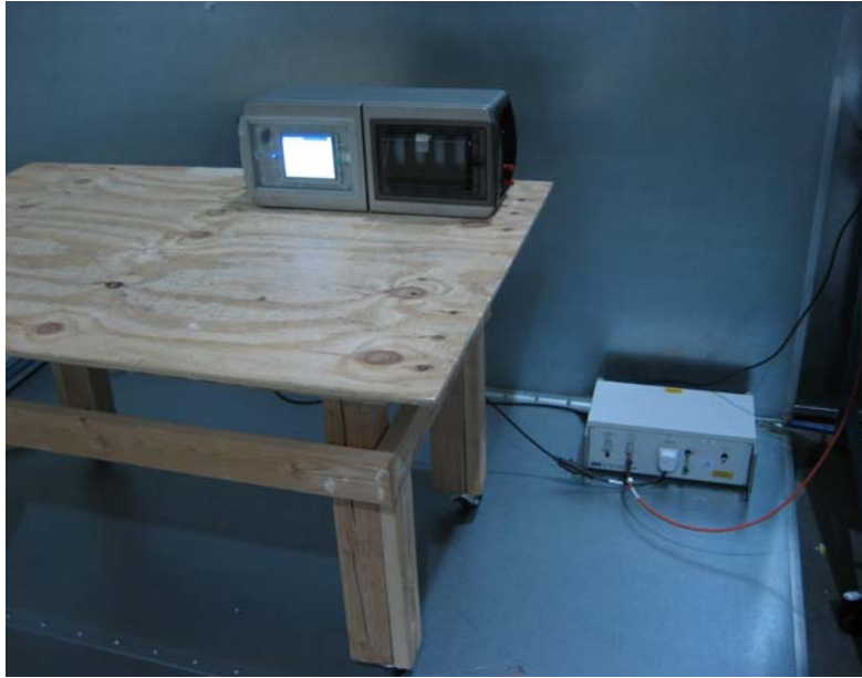
AC Line Conducted Emission Test Set-up Front View
