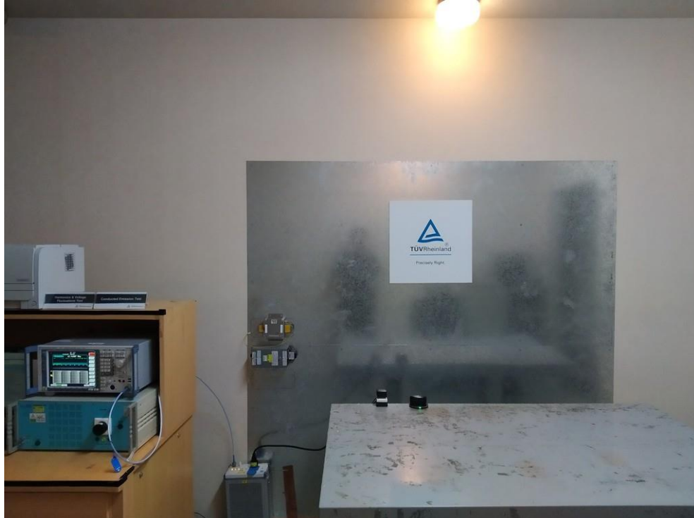
Picture 1: Test setup for Conducted Emission; 0.15 - 30 MHz
