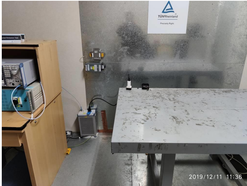
Photograph 9: Set-up for AC Mains (Front View)
