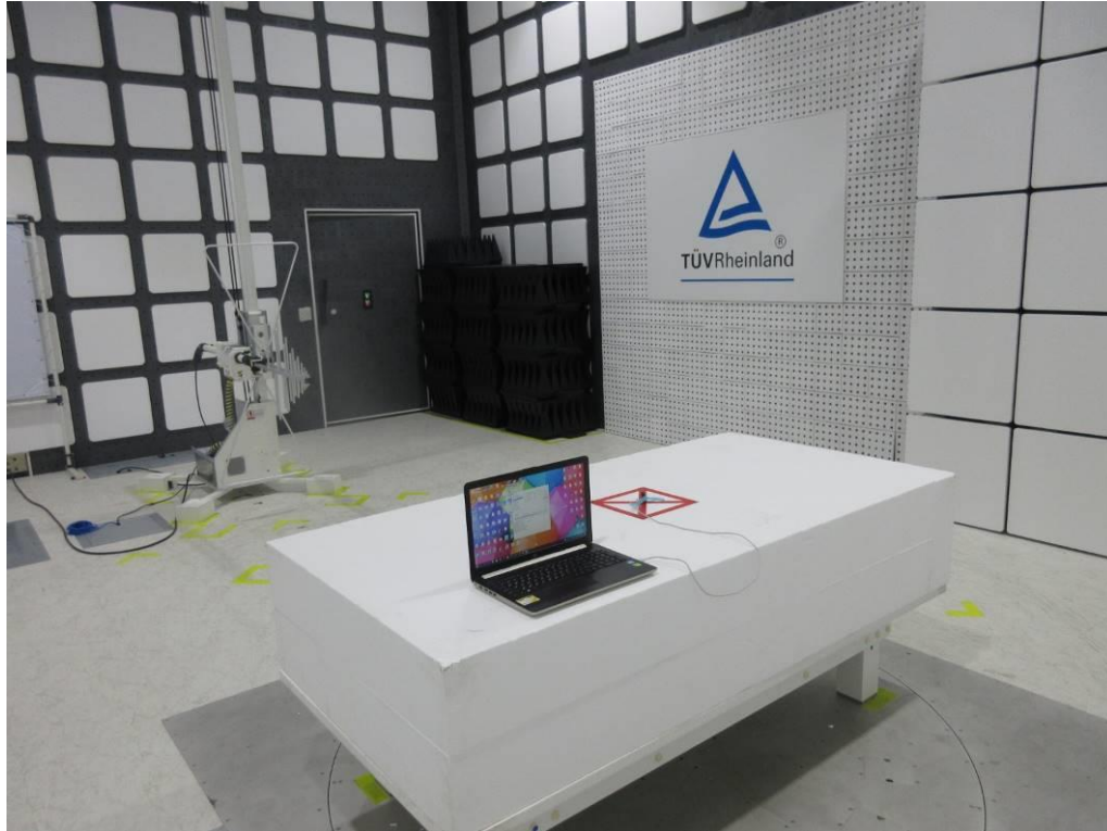
Photograph 3: Set-up for Spurious Emissions (Back View 1)
