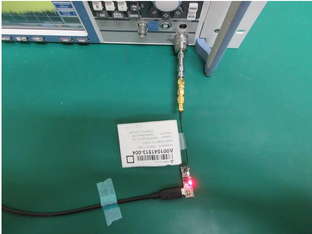
Photograph 7: Set-up for Conducted testing (View 1)
