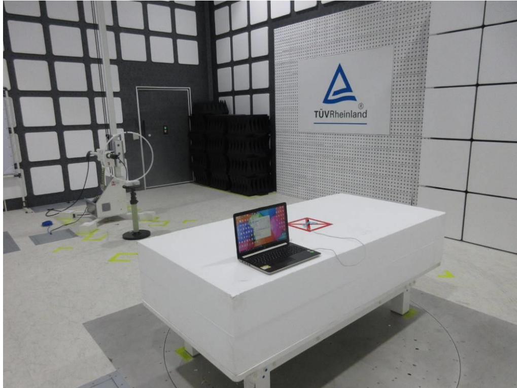
Photograph 5: Set-up for Spurious Emissions (Back View 3)
