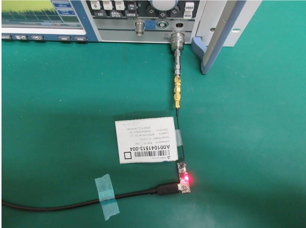
Photograph 7: Set-up for Conducted testing (View 1)
