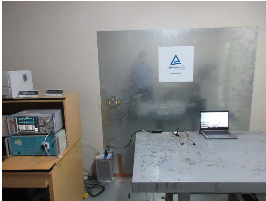
Photograph 7: Set-up for AC Mains (Front View)
