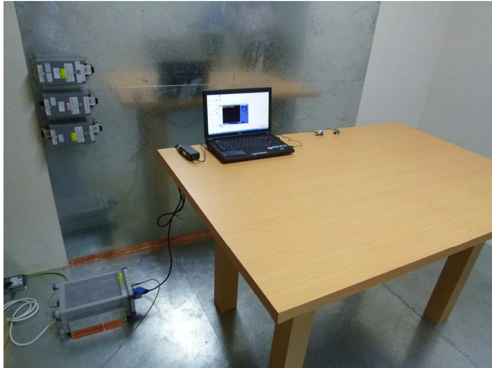
Photograph 4: Set-up for Mains Conducted Emissions (Back View)
