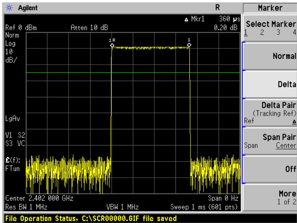
Single pulse @ GFSK mode Channel 17
