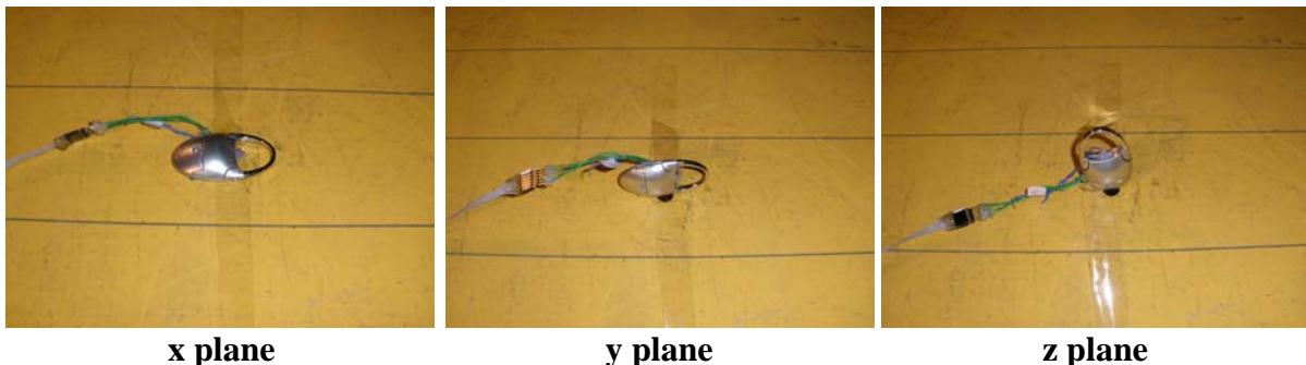
After verifying three axes, we found the maximum electromagnetic field was occurred at z-plane configuration. The final test data was executed under this configuration.
