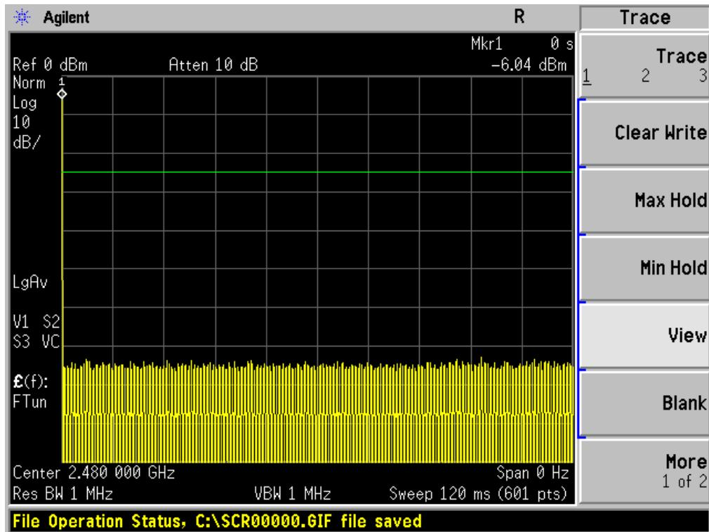
Single pulse @ GFSK mode Channel 37
