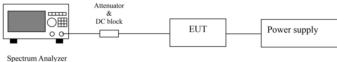
**Note:** The EUT was tested while in a continuous transmit mode and the data rates are 1 Mbps for GFSK. The EUT was tuned to a low, middle and high channel.
