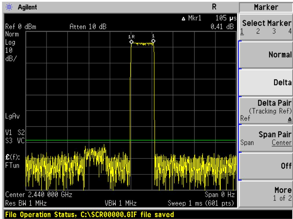
Single pulse @ GFSK mode Channel 39
