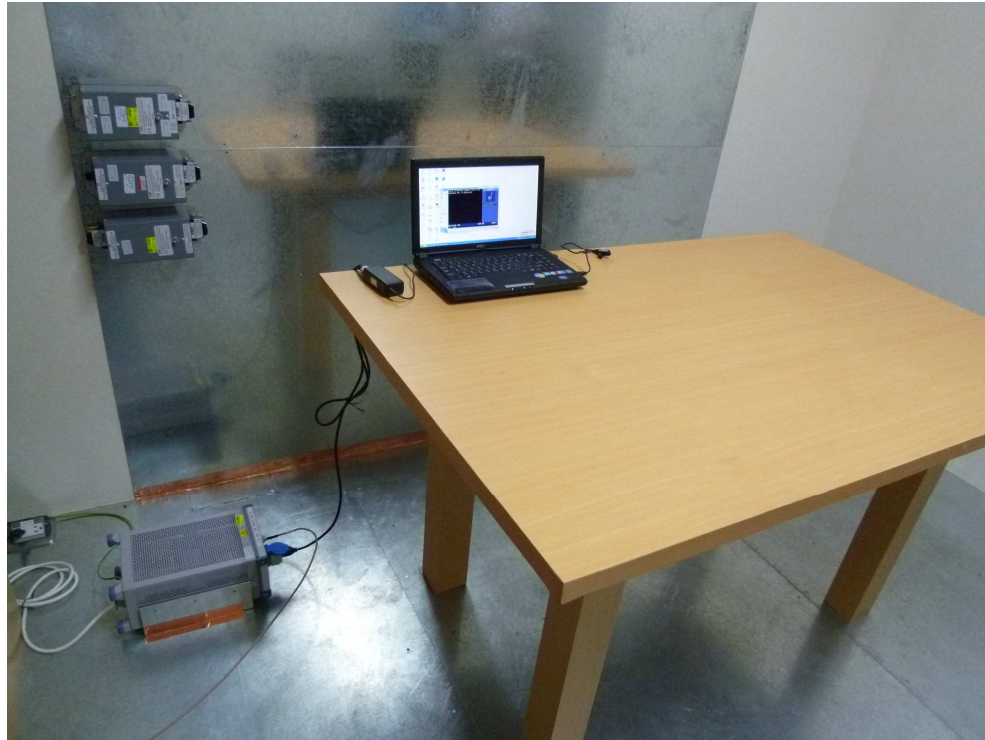
Photograph 4: Set-up for Mains Conducted Emissions (Back View)
