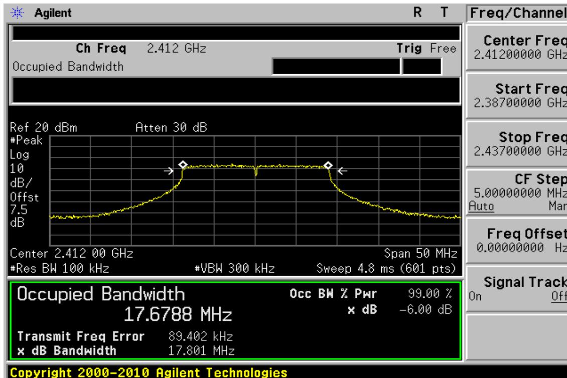
**6dB Band Width Test Data CH-Mid**
