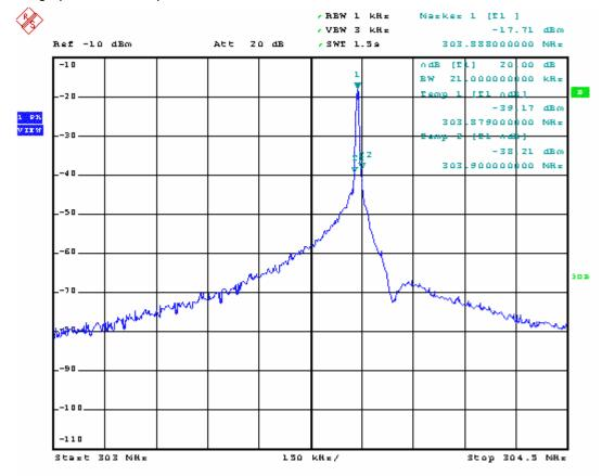
The results: The unit does meet the FCC Part 15C Section 15.231 requirements.
