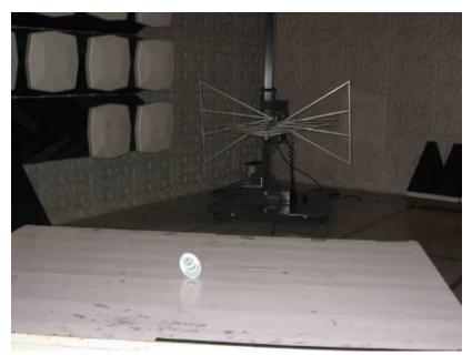
5.3.3 Photographs - Radiated Emission Test Setup in Chamber
