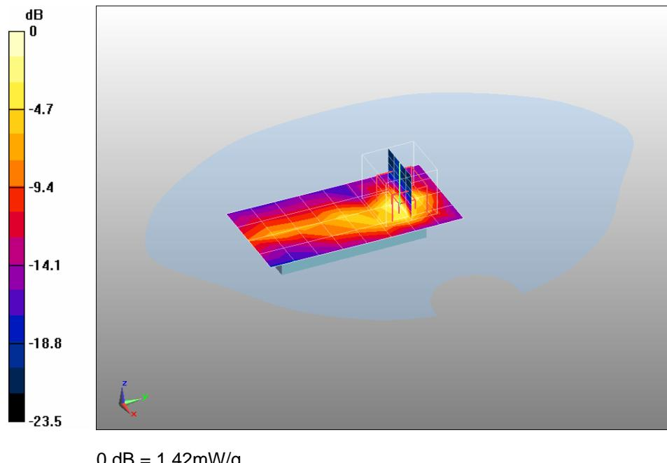
**802.11n(40MHz) EUT Bottom, Z-Axis Plot**
