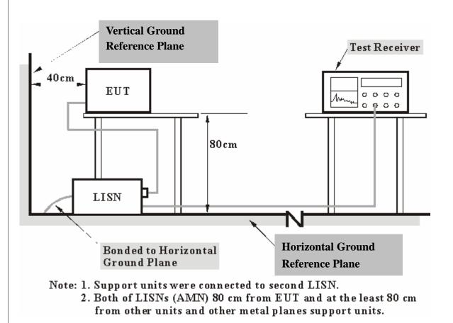
For the actual test configuration, please refer to the attached file (Test Setup Photo).
