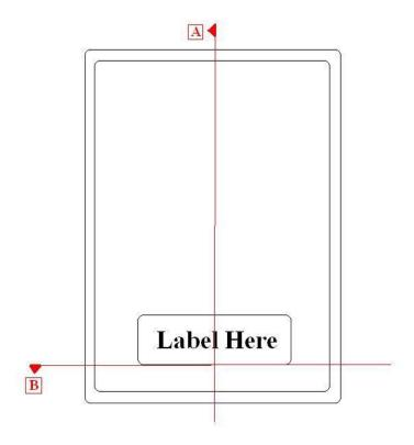
The FCC ID will be placed on the rear side of the equipment.
