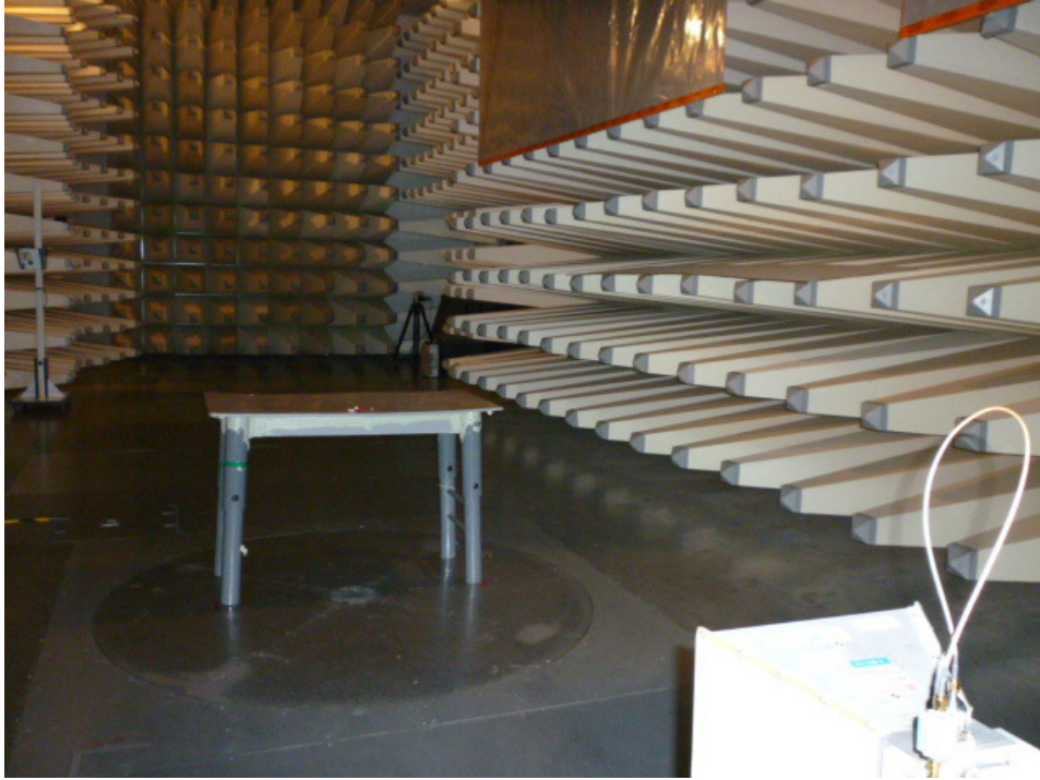
Setup for Radiated Emission
