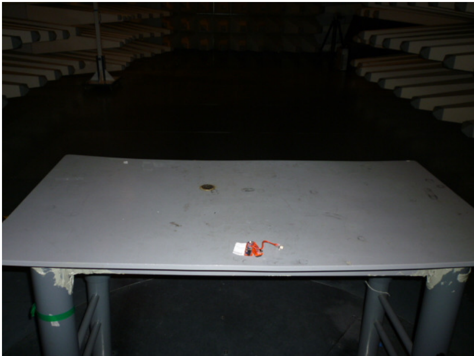
Setup for Radiated Emission
