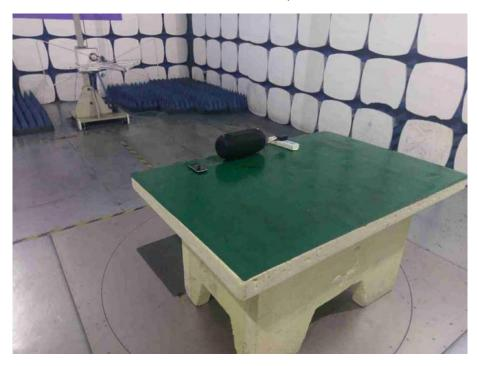
Radiated Emission Test, Above 1GHz
