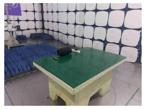
Radiated Spurious Emission Test, Below 1GHz
