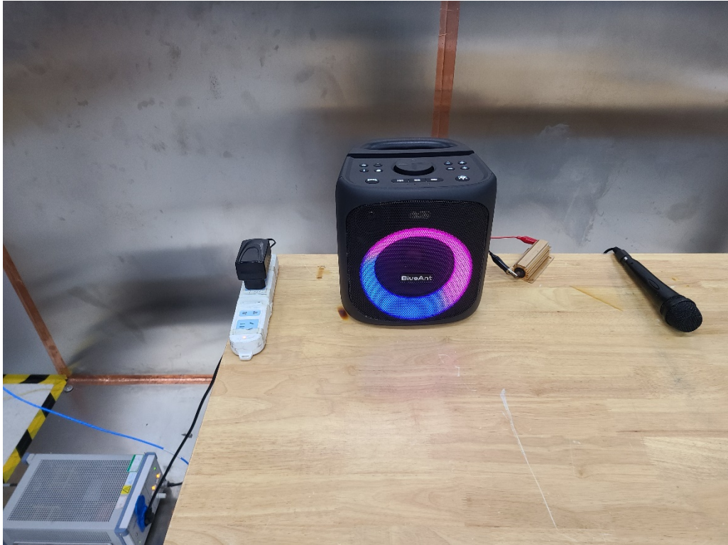
Photograph 3: Set-up for Conducted Emission on AC Mains
